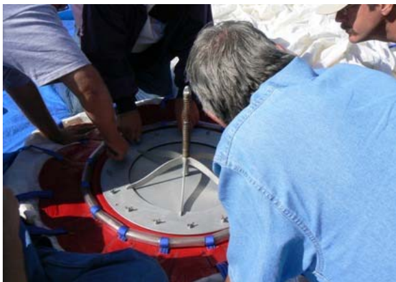
Installing a mechanical valve at the top of a gas balloon envelope.
