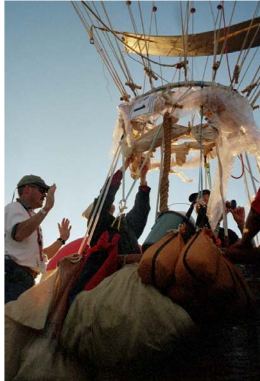
Austrian pilots Gerald Stürzlinger and Johann Fűrstner prepare to launch in the 2005 Gordon Bennett, as safety officer Matt Guthrie (left) takes “hands off.” Note the toggles attaching the envelope and basket to the load ring, the rain skirt tied around the load ring, and the orange sandbags tied to the side of the basket.
